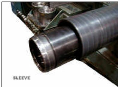
Install a sleeve (if available) on the threads of the section newly installed (Figure 25). Take the gland nut corresponding to the section that was just inserted and apply grease to it, specifically where the seal assembly is. Hydraulic oil soluble grease is strongly recommended.
