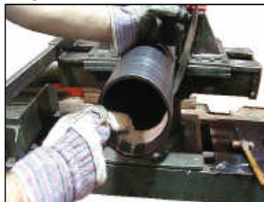
Insert the first section (next tube) in the base section and push it in approximately half way. Be sure to keep the section inserted as parallel as possible.
